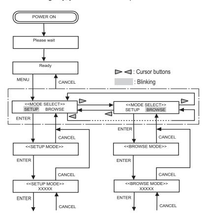
In the following way, you can use the test mode in addition to the setup mode and browse mode. To quit these modes, turn the power off.
